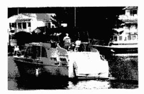
My good ship Ole," about to dock in the Chesapeake and Delaware canal. Note the partially enclosed steering station that can trap CO.
